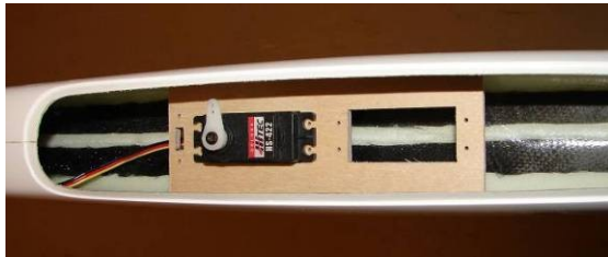
Use standard servos for Rudder and Elevator
