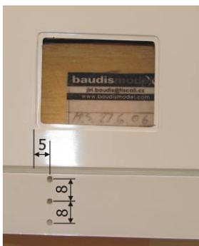
For horns drill holes 2mm
