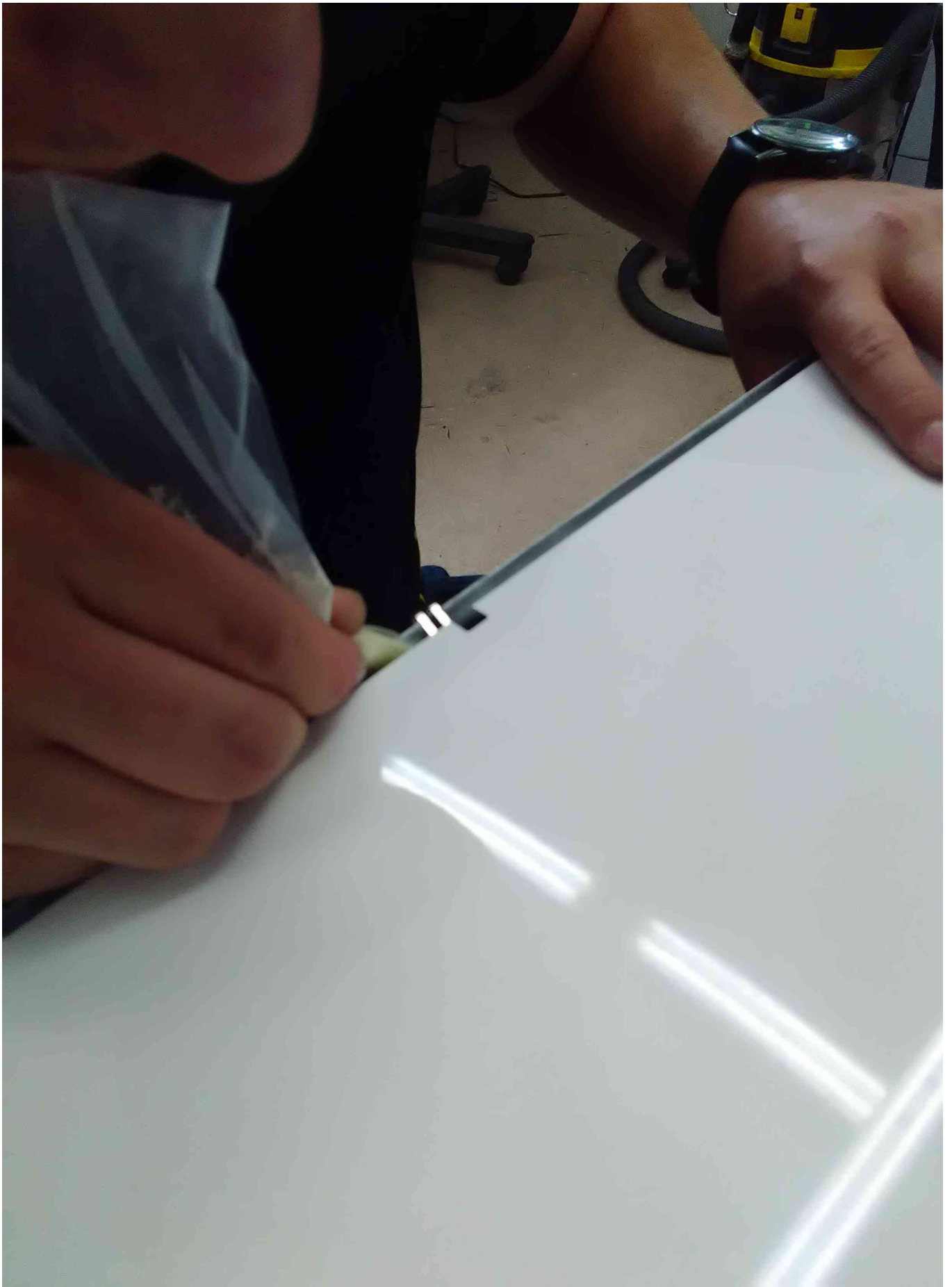
Apply epoxy to the lateral of the horns
