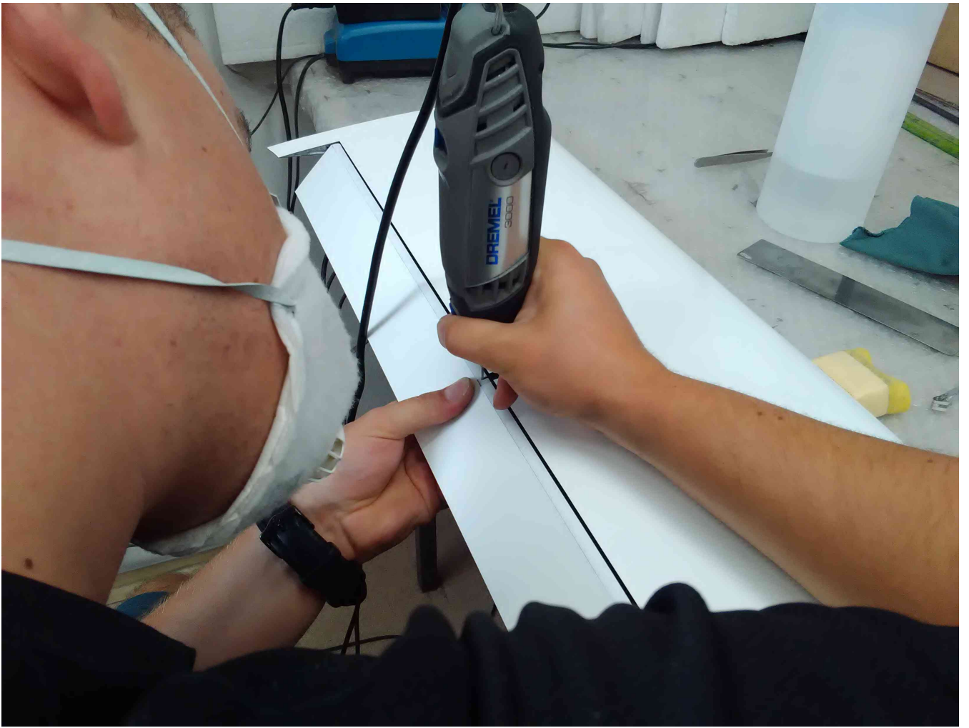
Cutting the flap's hinge feature
