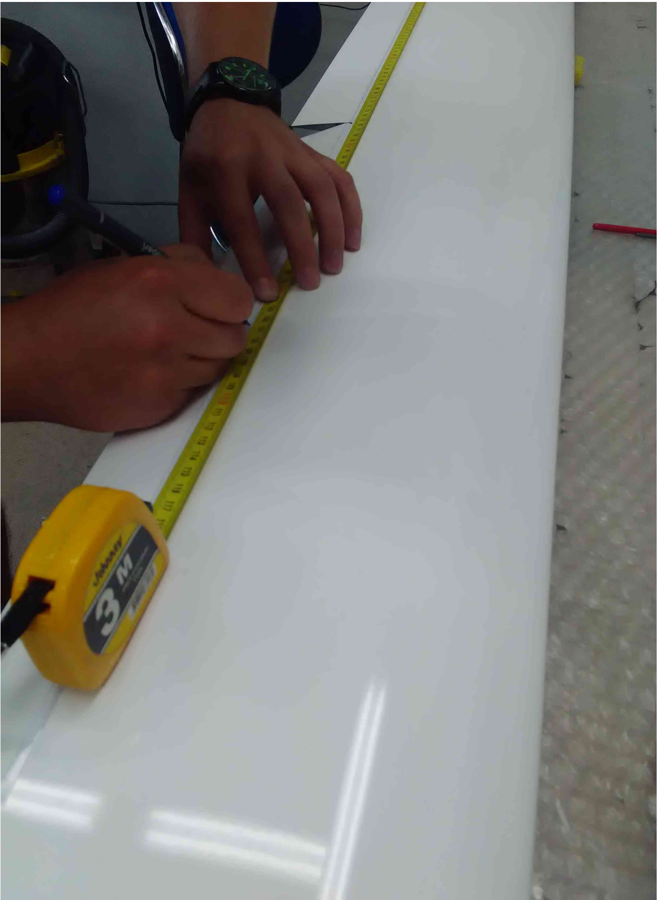
Measuring and making a mark in each horn position
