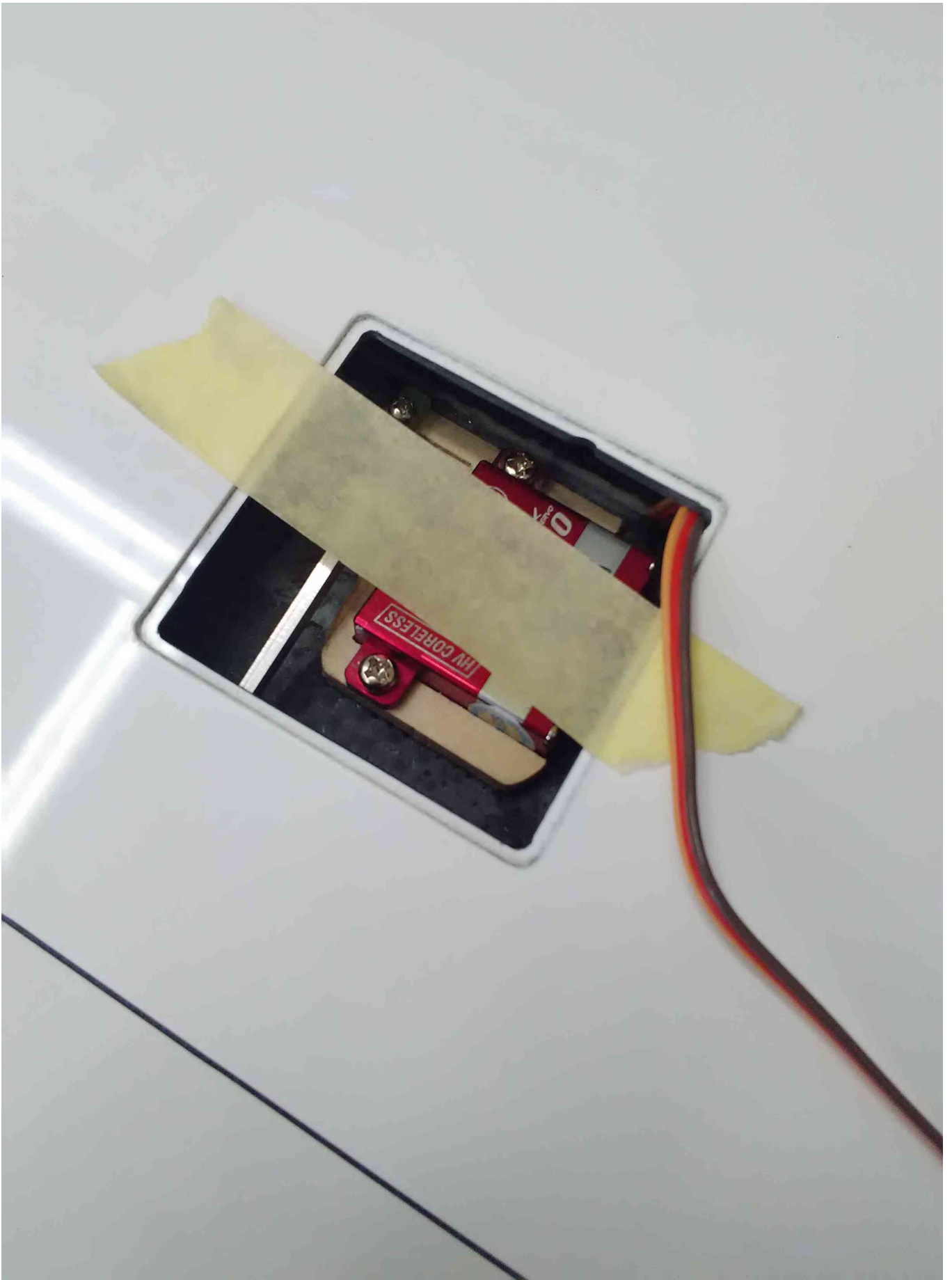
With a tape, fix them to not to fall off when you manipulate the wing
