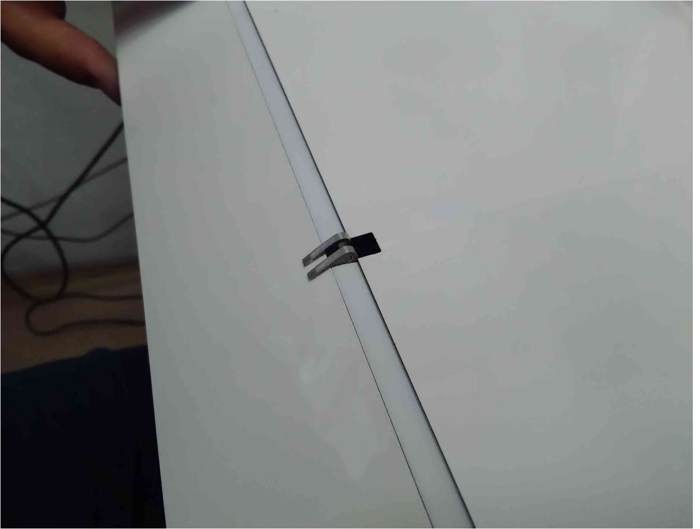
Checking if the hole in the wing is enough to accommodate the horn
