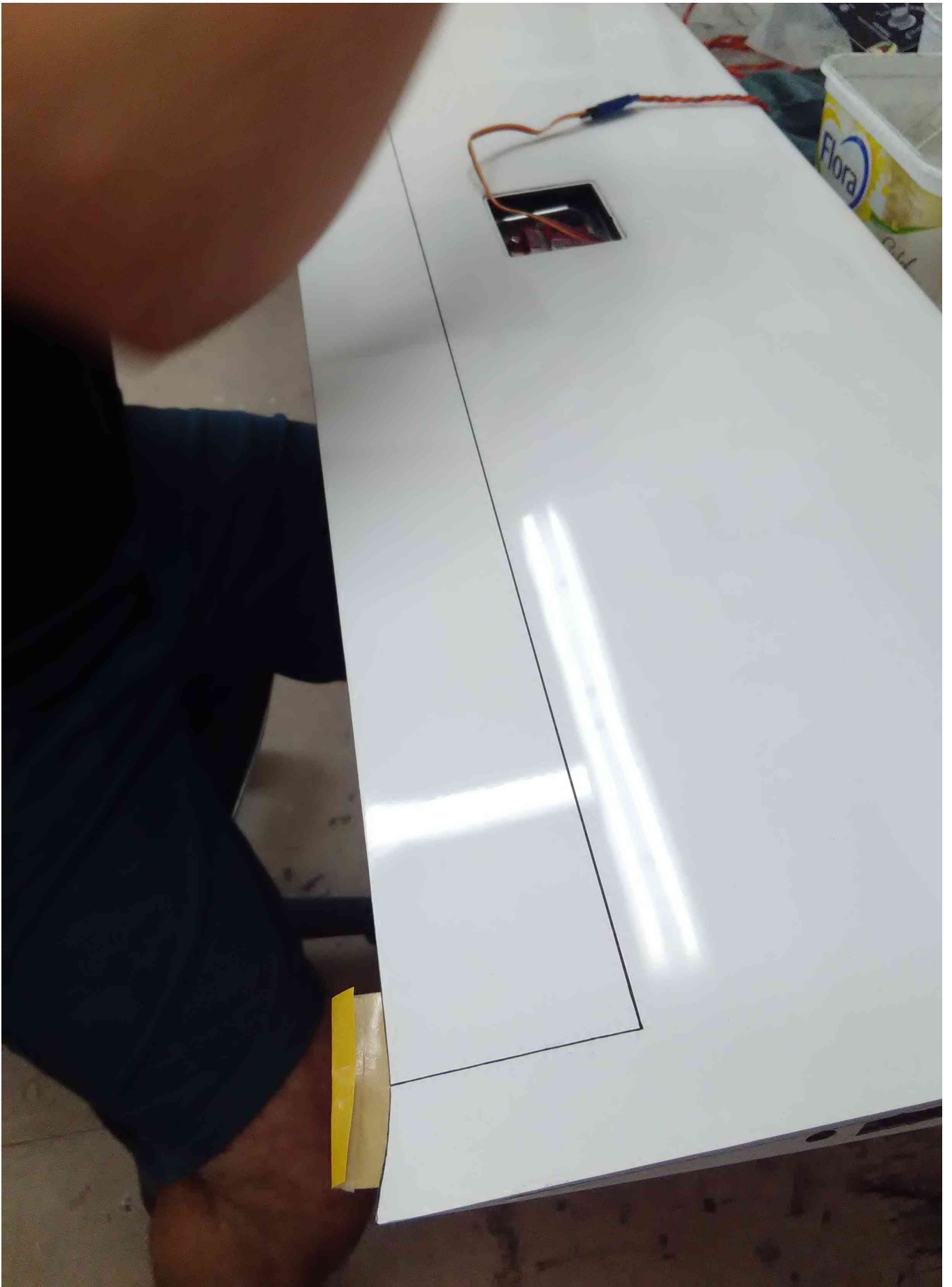
Tape the surface in its neutral position
