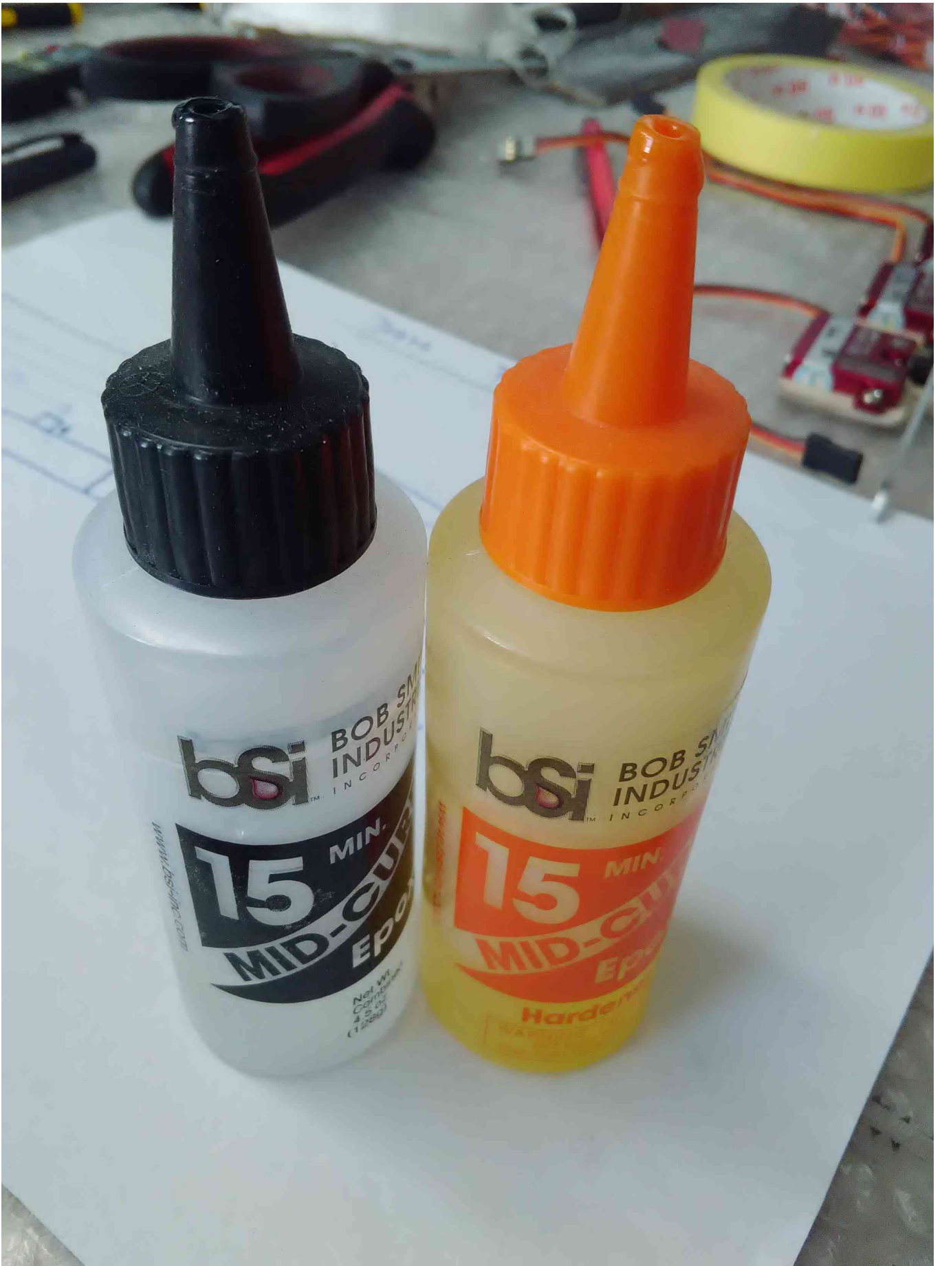
Prepare 15 min epoxy to temporary fix the horns
