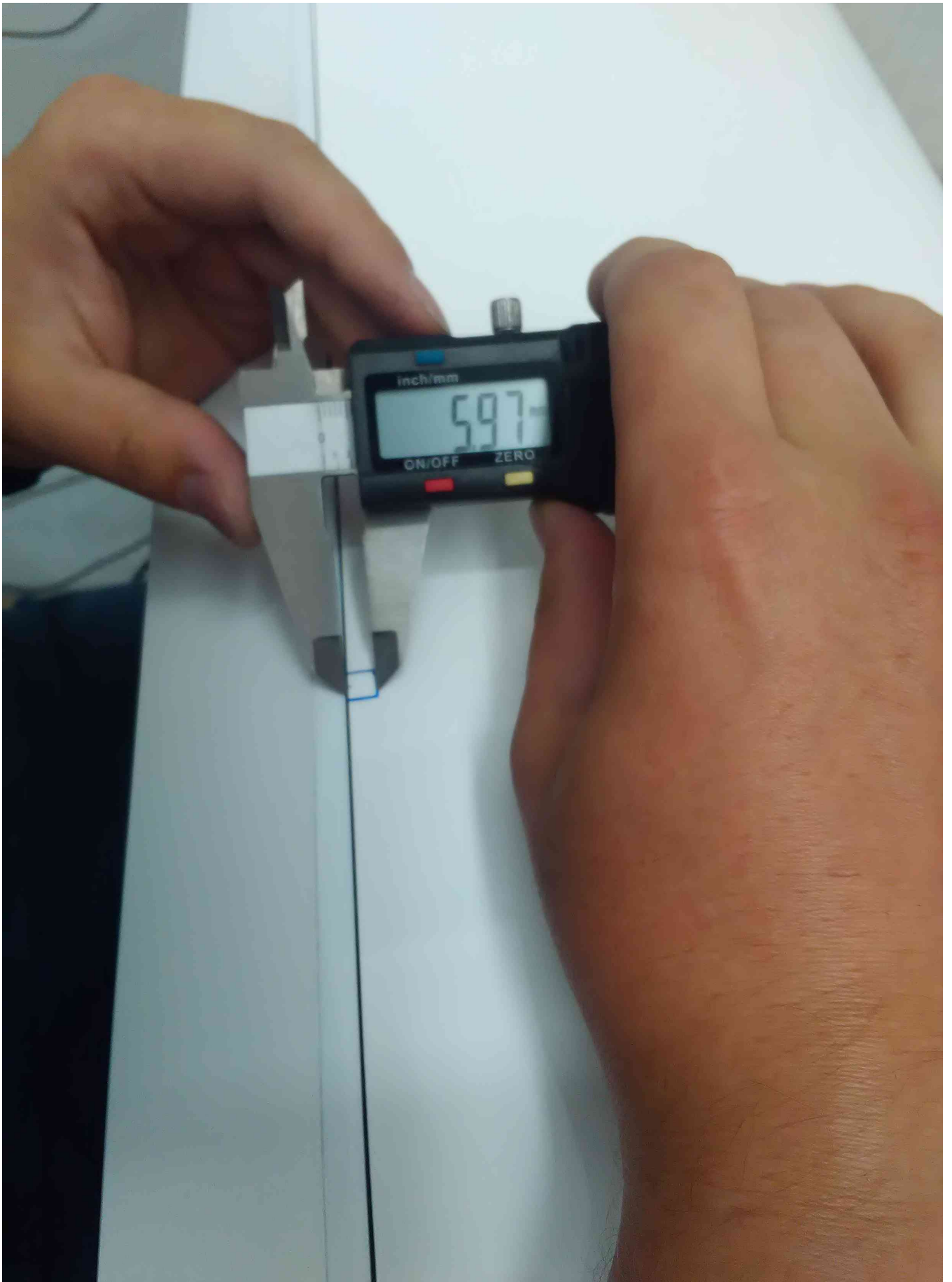
Marking 6mm exactly
