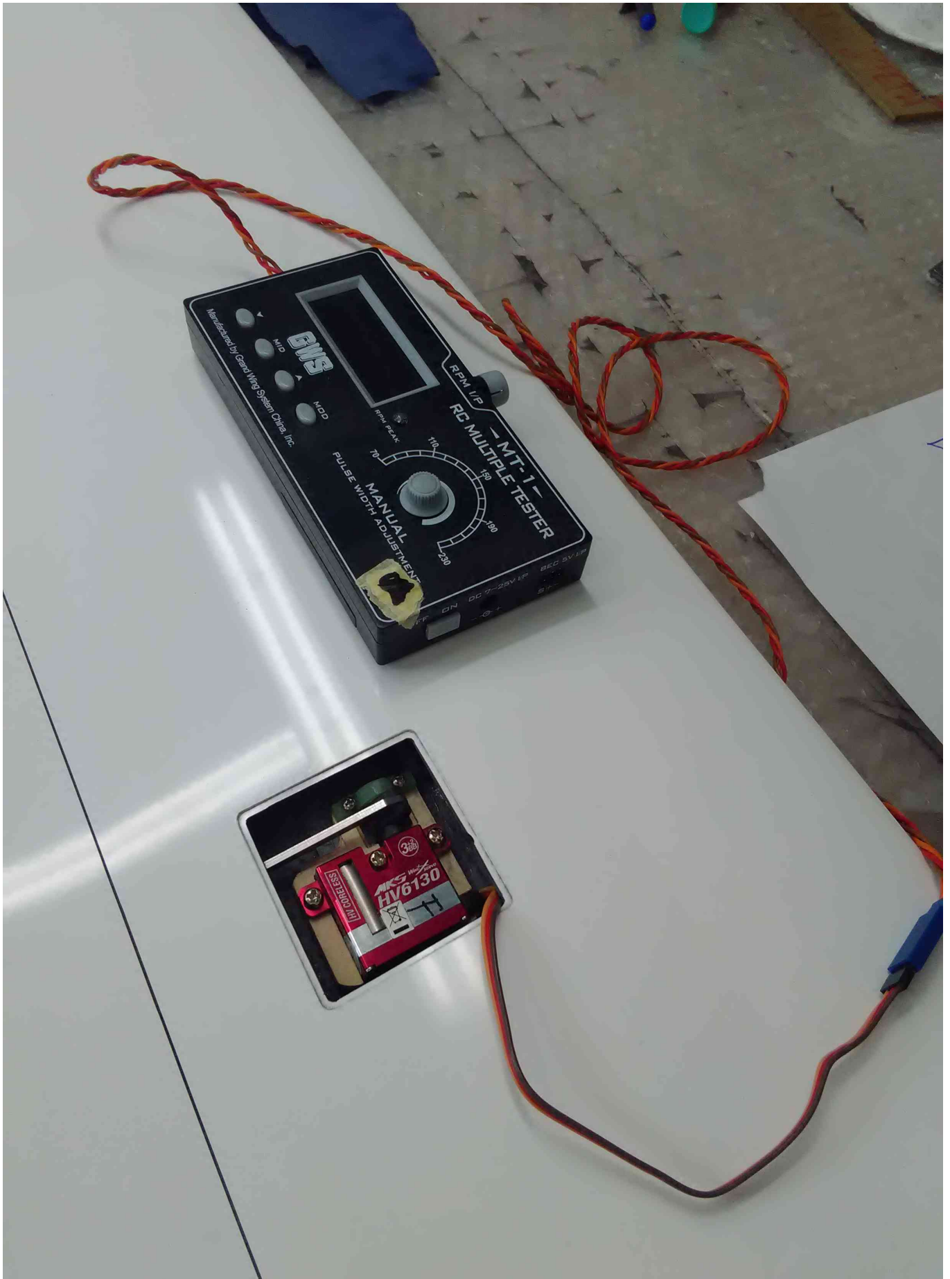
Use a servo driver to place the servos at specific position
