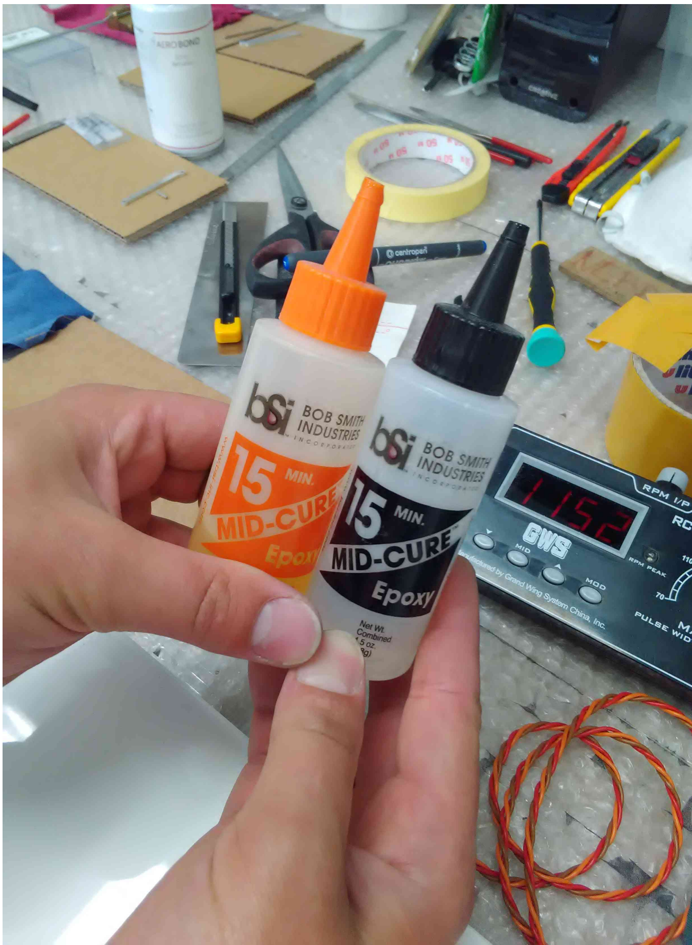
Prepare 15min epoxy to fix one servo at a time
