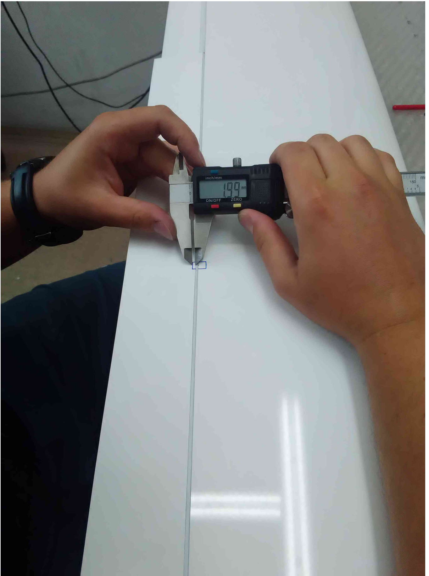
Marking the aileron cut limit
