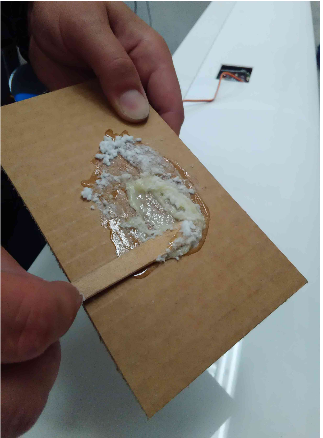
mix the epoxy with cotton to have a consistent glue
